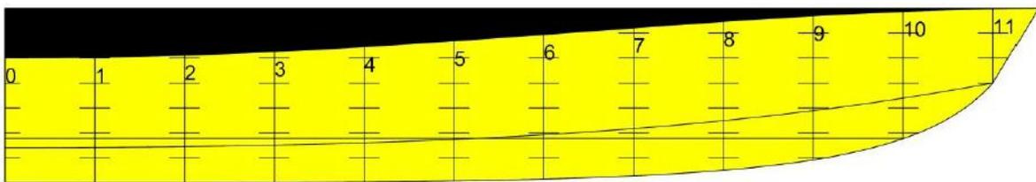
Figure 1 The picture shows an example of painting and marking for a hull model
